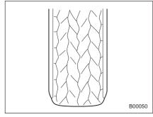
Roadholding is good, and steering is responsive. Rolling resistance is low, so fuel consumption is also lower. • Abnormally low tire pressure (tread worn at shoulders)
