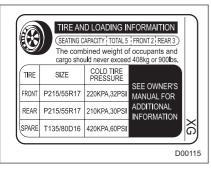
The vehicle placard shows original tire size, recommended cold tire inflation pressure on each tire at maximum loaded vehicle weight, seating capacity and loading information.
