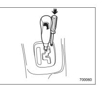
Insert the screwdriver into the hole.
