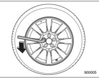
6. Loosen the wheel nuts using the wheel nut wrench but do not remove the nuts.
