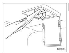
8. If the child restraint system requires a top tether, latch the hook onto the top tether anchor and tighten the top tether. See the "Top tether anchorages" for additional instructions.
