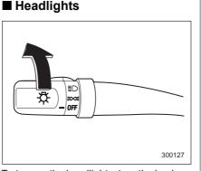
To turn on the headlights, turn the knob on the end of the turn signal lever.
