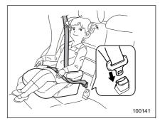
1. Place the booster seat in the rear seating position and sit the child on it. The child should sit well back on the booster seat.
