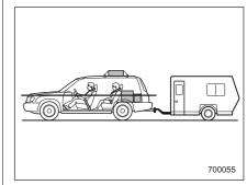
Owing to the self-leveling suspension, the vehicle body is adjusted to the proper position after several drive trips, even if the rear of the vehicle is lowered by loaded cargos or a coupled trailer.
