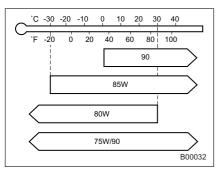
SAE viscosity No. and applicable temperature
