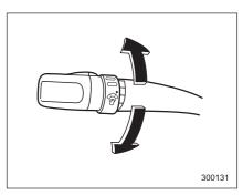
When the headlight switch is in the " $\exists O \Box \Xi$ " or " $\equiv \bigcirc$ " position, you can adjust brightness of the instrument panel illumination for better visibility. To brighten, turn the control dial upward. To darken, turn the control dial downward.
