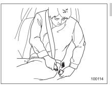
5. Insert the center seatbelt tongue plate in the center seatbelt buckle marked "CENTER" on the left-hand side until it clicks.
