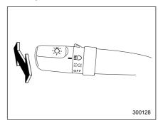
To change from low beam to high beam, push the turn signal lever forward. When the headlights are on high beam, the high beam indicator light "  $\equiv$  " on the instrument panel is also on.
