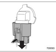
1. Disconnect the electrical connector from the bulb.
