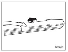
5. Align the claws of the metal support with the grooves in the rubber and slide the blade rubber assembly into the metal support until it locks.
