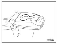
With the console top tipped toward the rear seat, it can be used as a cup holder.
