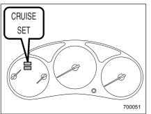
At this time, the " <sub>SET</sub> " indicator light is illuminated in the combination meter. The vehicle will maintain the desired speed.
