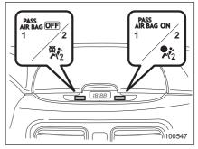
1) U.S.-spec. models 2) Canada-spec. models MR BAG ON or 2: Front passenger's frontal airbag ON indicator MR BAG OFF or 2: Front passenger's frontal airbag OFF indicator
