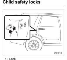
Each rear door has a child safety lock that prevents the doors from being opened even if the inside door handle is pulled. When the child safety lock lever is in the lock position, the door cannot be opened from inside regardless of the position of the inner door handle lock lever. The door can only be opened from the outside.
