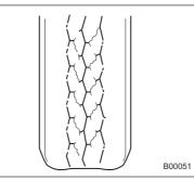
Rolling resistance is high, so fuel consumption is also higher. • Abnormally high tire pressure (tread worn in center)
