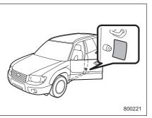
The load capacity of your vehicle is determined by weight, not by available cargo space. The maximum load you can carry in your vehicle is shown on the vehicle placard attached to the driver's side door pillar. It includes the total weight of the driver and all passengers and their belongings, any optional equipment such as a trailer hitch, roof rack or bike carrier, etc., and the tongue load of a trailer.
