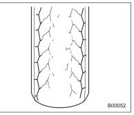
Ride comfort is poor. Also, the tire magnifies the effects of road-surface bumps and dips, possibly resulting in vehicle damage.
