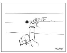
2. Locate the rear gate lock release lever behind the rear gate trim panel.
