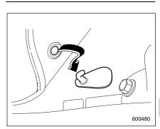
A retaining pin is located on the driver's side of the vehicle next to the fuel filler door release.
