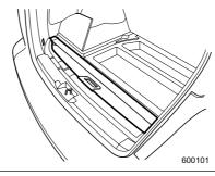
On models having a temporary spare tire, the cargo area cover can be stowed in under the cargo floor.
