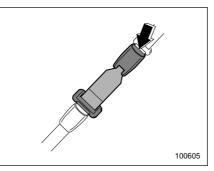
To connect the extender to the seatbelt, insert the tongue plate into the seatbelt buckle so that the "PRESS" signs on the buckle-release buttons of the extender and the seatbelt are both facing outward as shown in the diagram. You will hear a click when the tongue plate locks into the buckle.
