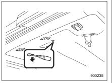
1. Remove the plug on the roof trim located to the rear of the moonroof by inserting the end of the flat-head screwdriver between the roof and plug and prying it off.
