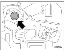
7. Remove the oil filter with an oil filter wrench.
