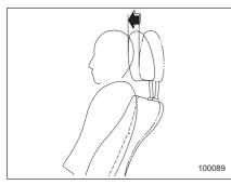
The front seats of your vehicle are equipped with active head restraints. They automatically tilt forward slightly in the event the vehicle is struck from the rear, decreasing the amount of rearward head movement and thus reducing the risk of whiplash. For maximum effectiveness the head restraint should be adjust so that the center of the head restraint is closest to the top of the occupant's ears.
