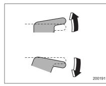
To open the passengers' windows, push the appropriate switch down and hold it until the window reaches the desired position.
