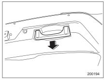
To close the rear gate, lower it slowly and push down firmly until the latch engages. The rear gate can be lowered easily if you pull down holding the recessed grip.
