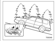
On an uphill grade, when the clutch pedal is depressed while the brake pedal is also depressed, braking power is maintained temporarily by the Hill holder when the brake pedal is released. The driver is therefore able to start the vehicle the same way as on a level grade, just using the clutch and accelerator pedal.
