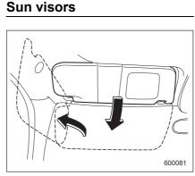
To block out glare, swing down the visors. To use the sun visor at a side window, swing it down and move it sideways.
