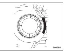
1. Remove the bulb cover, by turning it counterclockwise.
