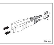
Pull out the fuse with the fuse puller.
