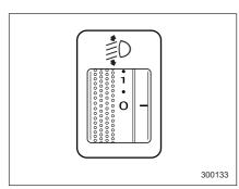
The 2.5XT has High-Intensity Discharge (HID) headlights on the low beam setting. The HID headlights generate more light than conventional halogen headlights. Therefore a driver of an oncoming vehicle may experience too much glare when your headlight beam height adjustment is high due to the vehicle carrying a heavy load.
