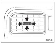
Move the tab up and down or right and left to adjust the flow direction.
