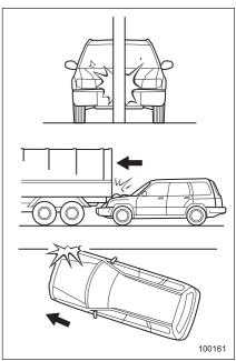
There are many types of collisions which might not necessarily require deployment
