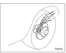
The right front disc brake and the right rear disc brake have audible wear indicators on the brake pads. If the brake pads wear close to their service limit, the wear indicator makes a very audible scraping noise when the brake pedal is applied.
