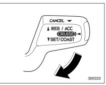
Push the control lever downward in the "SET/COAST" direction and hold it until the vehicle reaches the desired speed. Then, release the control lever. The vehicle speed at that moment will be memorized and treated as the new set speed.
