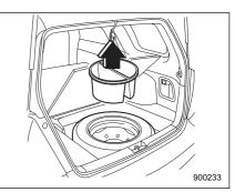
2. Remove the storage compartment bucket (Canada spec. non-turbo models).
