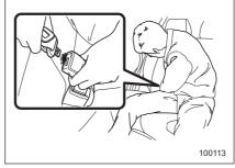
4. After confirming that the webbing is not twisted, insert the connector (tongue) attached at the webbing end into the buckle on the right-hand side until a click is heard. If the belt stops before reaching the buckle, return the belt slightly and pull it out more slowly. If the belt still cannot be unlocked, let the belt retract slightly after giving it a strong pull, then pull it out slowly again.
