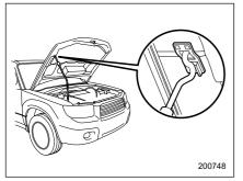
Lift up the hood, release the hood prop from its retainer and put the end of the hood prop into the slot in the hood. To close the hood:
