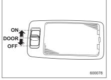
The dome light switch has three positions:
