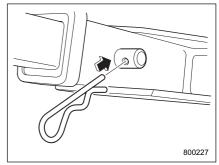
3. Insert the safety pin securely into the hitch pin.
