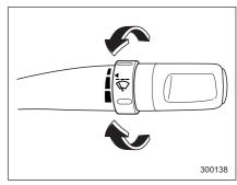
When the wiper switch is in the "  $\heartsuit$  " position, turn the dial to adjust the operating interval of the wiper.
