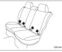
The lower anchorages (bars) are used for installing a child restraint system only on the rear seat window-side seating positions. For each window-side seating position, two lower anchorages are provided. Each anchor bar is located where the seat cushion meets the seatback.
