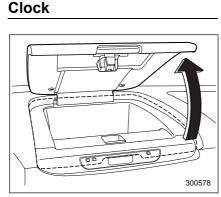
To adjust the clock, open the small article storage compartment in the dashboard with the vehicle parked in a safe place.
