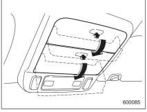
To open the console, push on the console lid lightly and the lid will automatically open.
