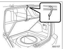
To keep the lid open, hang the hook provided on the backside of the lid on the rear
