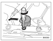
Before replacing the left-hand (batteryside) low- or high-beam light bulb, remove the screw that retains the windshield washer nozzle and tip the windshield washer nozzle sideways.
