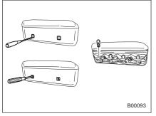
1. Remove the mounting screw covers by prying the edge with a flat-head screwdriver.
