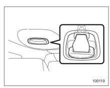
2. Allow the retractor to roll up the belt. You should hold the webbing end and guide it back into the retractor while it is rolling up. Neatly store the tongue plates in the recess on the ceiling and then insert the connector (tongue) plate into the slot located at the front of the recess.
