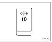
The front fog lights operate only when the headlights are on low beam. Push the front fog light button to turn the front fog lights on.
