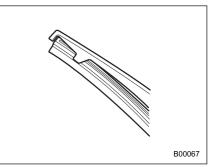
Securely lock the end of the plastic support as shown in the illustration. If the rub-
