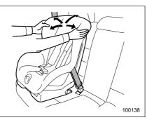
6. Before having a child sit in the child restraint system, move it back and forth and right and left to check if it is firmly secured. Sometimes a child restraint can be more firmly secured by pushing it down into the seat cushion and then tightening the seatbelt.
