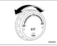
This dial is used to set the desired interior temperature. With the dial set to your desired temperature, the system automatically adjusts the temperature of air supplied from the outlets such that the desired temperature is achieved and maintained. If the dial is turned fully counterclockwise, the system gives maximum cooling performance. If the dial is turned fully clockwise, the system gives maximum heating performance.
