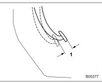
1) Non-turbo models: 0.39 – 0.79 in (10 – 20 mm) Turbo models: 0.12 – 0.51 in (3 – 13 mm)
