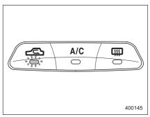
**ON position (Recirculation):** Interior air is recirculated inside the vehicle. Push the air inlet selection button to the ON position. The indicator light will come on. Place the air inlet selection button to the ON position for fast cooling with the air conditioner or when driving on a dusty road.
