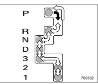
With the brake pedal depressed, move the lever along the gate.
