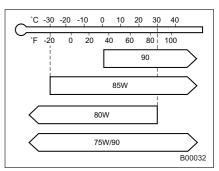
SAE viscosity No. and applicable temperature
