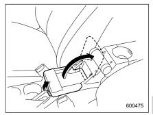
Raise the console top to the vertical position or tip it toward the rear seat. Then, pull up the lock button of the console box and open the lid.
