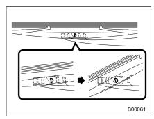
2. Turn the wiper blade assembly counterclockwise.
