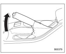
Check the parking brake stroke according to the maintenance schedule in the "Warranty and Maintenance Booklet". When the parking brake is properly adjusted, braking power is fully applied by pulling the lever up seven to eight notches gently but firmly (approximately 44 lbs, 196 N, 20 kg). If the parking brake lever stroke is not within the specified range, have the brake system checked and adjusted at your SUBARU dealer.
