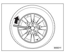
13.Use the wheel nut wrench to securely tighten the wheel nuts to the specified torque, following the tightening order in the illustration.
