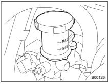
Check the fluid level on the outside of the reservoir. If the level is below "MIN" level mark, add the recommended clutch fluid to "MAX" level mark.
