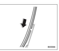
7. Align the claws of the plastic support with the grooves in the blade rubber assembly, then slide the blade rubber assembly into place.
