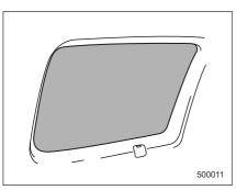
The antenna is printed on the inner surface of the left side rear quarter window glass.
