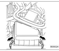
1. Unsnap the two clamps holding the air cleaner case cover.
