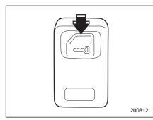
5. Before the electronic tone stops sounding, push the lock side of the power door lock switch the same number of times as the leftmost digit of the transmitter code. For example, push the lock switch eight times if the leftmost digit of the code is 8.
