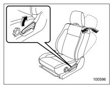
Pull the reclining lever up and adjust the seatback to the desired position. Then release the lever and make sure the seatback is securely locked into place. The seatback placed in a reclined position can spring back upward with force when released. When operating the reclining lever to return the seatback, hold it lightly so that it may be raised back gradually.
