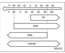
SAE viscosity No. and applicable temperature
