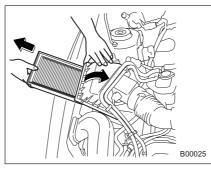
2. Open the air cleaner case cover and remove the air cleaner element.
