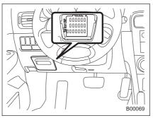
One is located under the instrument panel behind the cover on the driver's seat side. To remove the cover, pull it out.
