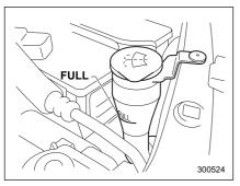
Remove the washer tank filler cap, then check the fluid level indicated by the level gauge (attached to the inside of the cap). If the level is near the "Low" mark, add fluid until it reaches the "Hi" level on the level gauge or the "Full" mark on the tank.
