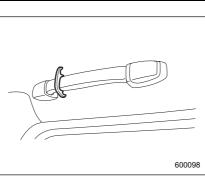
The coat hook is attached to the rear left passenger's hand grip.
