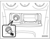
The cigarette lighter operates only when the ignition switch is in the "ON" and "ACC" positions.
