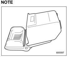
Particles of ash and tobacco will accumulate around the hinges of the ashtray's inner lid. Clean them off using a toothbrush or other narrow-ended implement.
