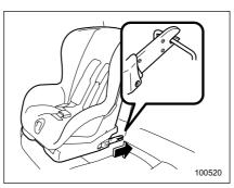
2. While following the instructions supplied by the child restraint system manufacturer, connect the lower hooks onto the lower anchorages located at " S " marks on the bottom of the rear seatback. When the hooks are connected, make sure the adjacent seatbelts are not caught.
