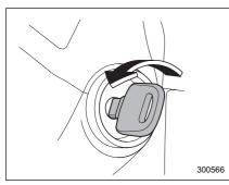
The key can be turned from "ACC" to "LOCK" only when the selector lever is in the "P" position.
