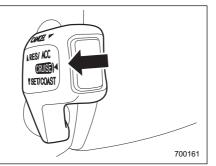
• Pull the control lever in the "CANCEL" direction (if so equipped).
