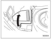
The jack handle is stowed under the rearleft and center lids in the cargo area. For how to use the jack, refer to the "Flat tires" section in this chapter.
