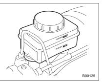
Check the fluid level monthly. Check the fluid level on the outside of the reservoir. If the level is below "MIN", add the recommended brake fluid to "MAX". Use only brake fluid from a sealed container.
