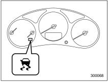
This single light has the function of indicating malfunctions in the Vehicle Dynamics Control system and the function of indicating that the Vehicle Dynamics Control system is not operating. It comes on in the event of a malfunction in the system and is illuminated whenever the system is not operating.
