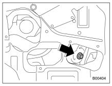
5. Drain out the engine oil by removing
