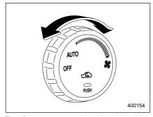
The fan operates only with the ignition switch in the ON position. The fan speed control dial is used to select the AUTO (automatic control) mode or to select the desired fan speed. The dial's positions and their functions are as follows: **OFF:** The fan does not operate.
