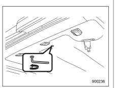
2. Insert a hex-headed wrench in the end of the motor shaft.
