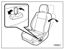
To adjust the angle of the seatback, move the control switch forward or backward.
