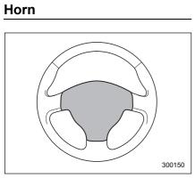
To sound the horn, push the horn pad.
