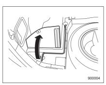
To take out the jack handle: Open the rear-left and center lids in the cargo area by pulling their tabs.
