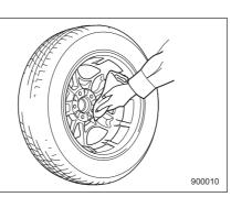
10.Before putting the spare tire on, clean the mounting surface of the wheel and hub with a cloth.
